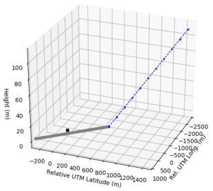
The physical characteristics of the runway (gray stripe) and the chosen location for the installation of the LiDAR device (black point) lead to the tridimensional modelling of the glide path (blue line)
