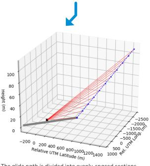
The glide path is divided into evenly-spaced sections. By leveraging the LiDAR's scanning flexibility, the beams (in red) that can measure wind speed at these sections are computed.
