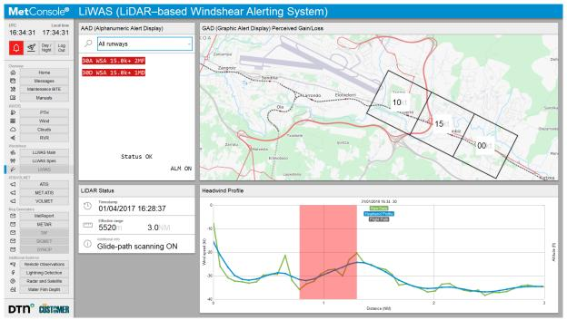
LiWAS Screen displaying a windshear alert in MetConsole.
