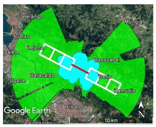
Comparison between a typical LLWAS range (blue) vs. LiWAS range (green), using an ASTER GDEM simulation. For reference, the runway (red line) and the ARENA (white grid) are drawn. Depending on the configuration of the physical runways, it may be recommended the installation of one or various LiDAR devices to achieve the best measurement accuracy and coverage area.
