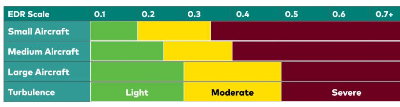
How the different levels of EDR relate to qualitative categorical turbulence measurements for different types of aircraft.
